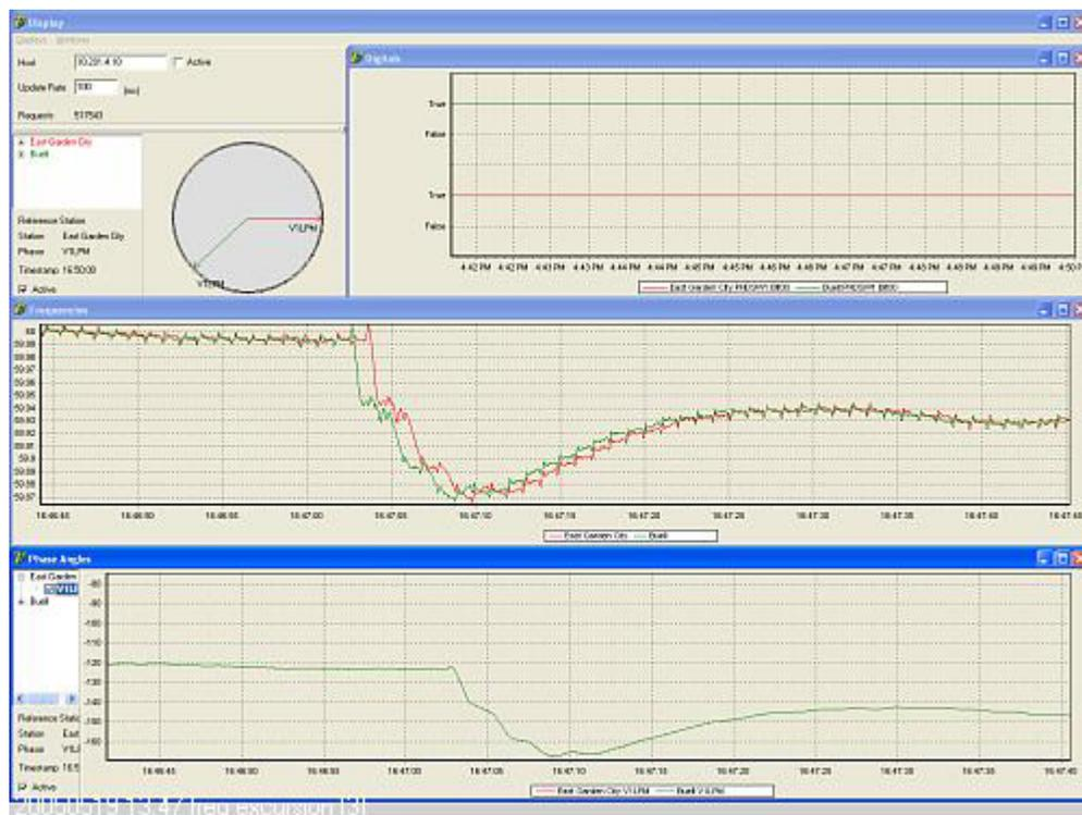
Fig. 8. Industrial view of frequency event plus local pulsed load.
