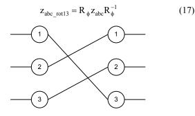
Fig. 17. Conductor rotation with Position 1 going to Position 3
