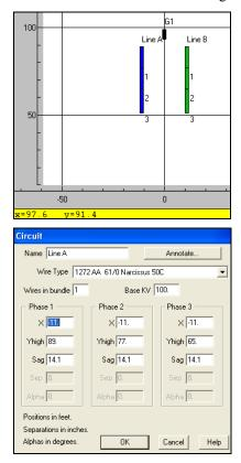
Fig. 1. ASPEN Line Constants Program screen captures showing the physical configuration of two circuits in a single right of way
