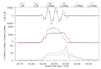
Fig. 10. Negative-sequence current and voltage magnitudes for Event 3
