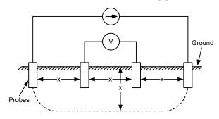
Fig. 4. Wenner four-point method for measuring ground resistivity
