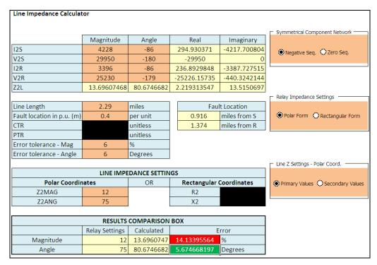
Fig. 11. Line impedance calculator created in Microsoft Excel
