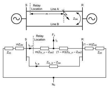
Fig. 7. System configuration and zero-sequence network for two mutually coupled lines
