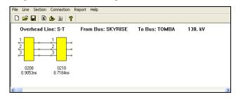
Fig. 2. ASPEN Line Constants Program screen capture showing two line sections with different tower configurations
