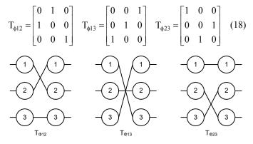
Fig. 18. Three cases of conductor twisting
