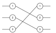
Fig. 16. Conductor rotation with Position 1 going to Position 2
