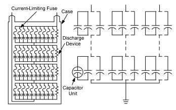
Fig. 2. Internally fused unit in a wye bank
