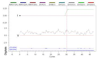
Fig. 4. Double-wye bank, single element failure
