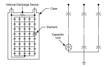
Fig. 1. Fuseless unit in a wye-connected bank
