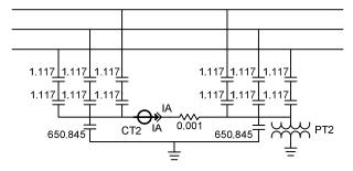
Fig. 3. Double-wye capacitor grounded bank
