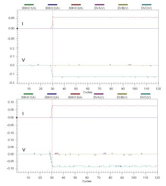
Fig. 13. C-type filter bank, single element failure in main (upper graph) and tuning bank (lower graph)
