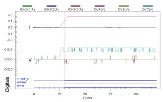
Fig. 9. Double H bank, single element failure
