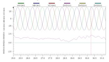
Fig. 7. Double-wye bank, primary voltage and differential voltage before and after a single element failure
