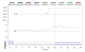
Fig. 5. Double-wye bank, two elements failed
