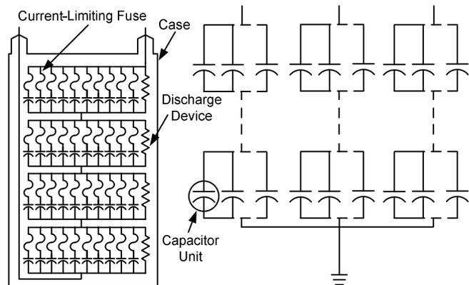
Fig. 2. Internally fused unit in a wye bank
