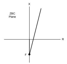
Fig. 26. A series capacitor in front of the relay plots as a negative reactance on the ZBC plane, which gives the idea that a directional element will not operate for a fault beyond the capacitor.
