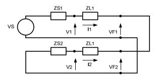
Fig. 2. Symmetrical component network for a bolted phase-to-phase fault.
