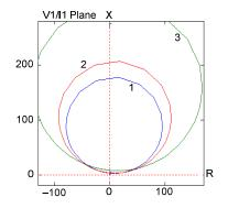
Fig. 22. Power swing trajectories for a balanced power swing (Trajectory 1) and for unbalanced power swings, using line-side (Trajectory 2) and bus-side (Trajectory 3) voltage to calculate V1.
