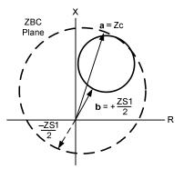
Fig. 7. BC polarized mho element characteristic for reverse BC faults.
