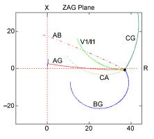
Fig. 11. Loci of the impedances measured by all distance elements at Bus S for AG faults with RF varying from  $RF = \infty$  (shown by the point) to RF = 0 (forward load flow). The labels refer to distance elements.
