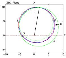
Fig. 9. BC element characteristics for different values of ILD/I2. Characteristic 0 is for no load; Characteristic 1 is for ILD/I2 = 0.3, arg (ILD) =  $0^{\circ}$ , arg (I2) =  $-85^{\circ}$ ; Characteristic 2 is for ILD/I2 = 0.3, arg (ILD) =  $180^{\circ}$ , arg (I2) =  $-85^{\circ}$ ; Characteristic 3 is for ILD/I2 = 1, arg (ILD) =  $0^{\circ}$ , arg (I2) =  $-5^{\circ}$ ; and Characteristic 4 is for ILD/I2 = 1, arg (ILD) =  $180^{\circ}$ , arg (I2) =  $-5^{\circ}$ .
