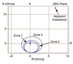
Fig. 29. ZBG plane representation of the external BG fault (Section 1 in Fig. 28).
