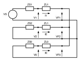
Fig. 8. Symmetrical component network for a phase-to-phase-to-ground fault.
