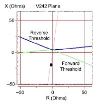
Fig. 23. Negative-sequence directional element characteristics.
