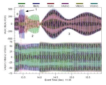
Fig. 28. Oscillogram recorded by an unfaulted 115 kV line relay. Section 0 is the prefault condition; Section 1 is an external BG fault followed by an incorrect single-pole trip; Section 2 is an unbalanced power swing during the B-phase open period; and Section 3 is a balanced power swing after faulted line tripping and unfaulted line B-phase reclosing.
