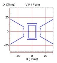
Fig. 18. Power swing detection and load-encroachment element characteristics.
