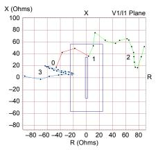
Fig. 31. Positive-sequence plane representation of the event shown in Fig. 28. Point 0 is the prefault condition; Point 1 is a BG fault; Trajectory 2 is an unbalanced power swing (B-phase open); and Trajectory 3 is a balanced power swing.
