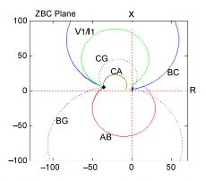
Fig. 14. Loci of the impedances measured by all distance elements at Bus R for BC faults with RF varying from  $RF = \infty$  (shown by the point) to RF = 0 (reverse load flow). The labels refer to distance elements.
