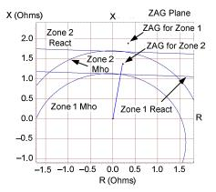
Fig. 17. Different k0 settings make Zone 1 and Zone 2 elements measure different impedances for phase-to-ground faults.
