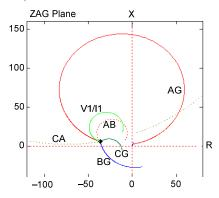
Fig. 12. Loci of the impedances measured by all distance elements at Bus R for AG faults with RF varying from  $RF = \infty$  (shown by the point) to RF = 0 (reverse load flow). The labels refer to distance elements.
