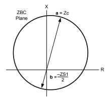
Fig. 4. BC polarized mho element characteristic for forward BC faults.
