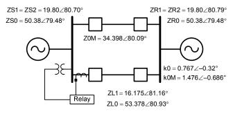
Fig. 16. Example 230 kV system that includes a double-circuit line.
