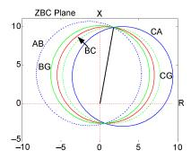
Fig. 5. BC element characteristics for different types of forward faults. The labels refer to fault types.
