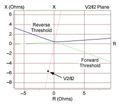
Fig. 30. Negative-sequence plane representation of the external BG fault (Section 1 in Fig. 28).
