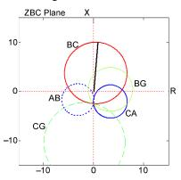
Fig. 6. Characteristics of all the distance elements on the ZBC plane for a forward BC fault. The labels refer to distance elements.
