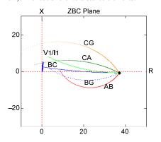
Fig. 13. Loci of the impedances measured by all distance elements at Bus S for BC faults with RF varying from  $RF = \infty$  (shown by the point) to RF = 0 (forward load flow). The labels refer to distance elements.
