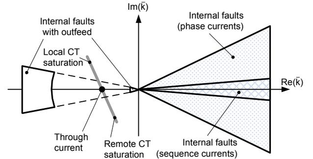
Fig. 3. Power system events on the Alpha Plane.
