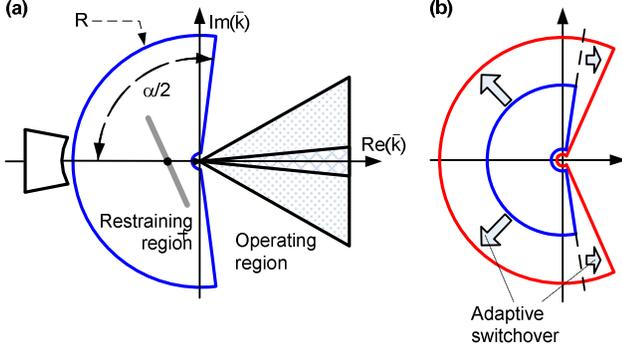
Fig. 5. Alpha Plane differential element operating characteristic (a); adaptive Alpha Plane characteristic with normal and extended security settings (b).
