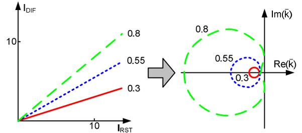
Fig. 6. Mapping a single-slope characteristic into the current-ratio plane.
