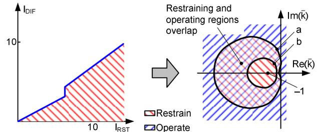
Fig. 8. Mapping a dual-slope characteristic into the current-ratio plane. The operating and restraining regions overlap on the Alpha Plane.
