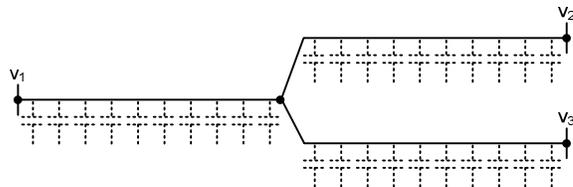
Fig. 29. Distributed capacitance three-terminal line model.
