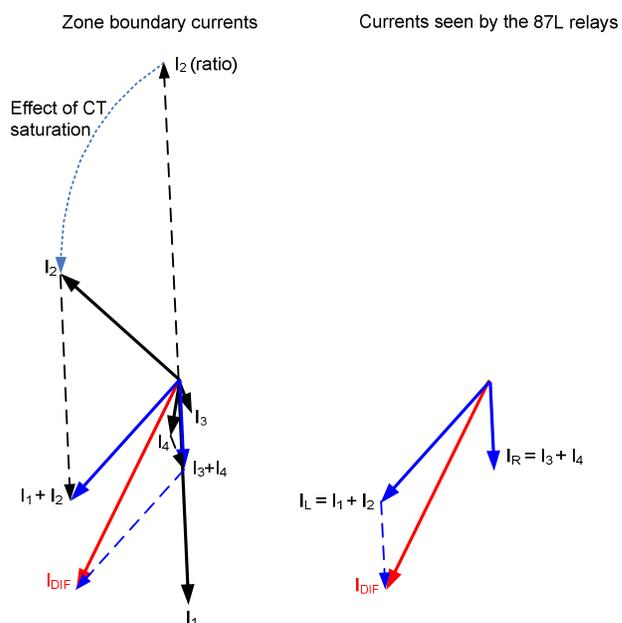
Fig. 11. Current phasors in Example 2, assuming the 87L relays are connected to paralleled CTs.
