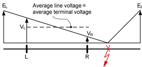
Fig. 33. During external faults, the average terminal voltage and the average line voltage are the same.
