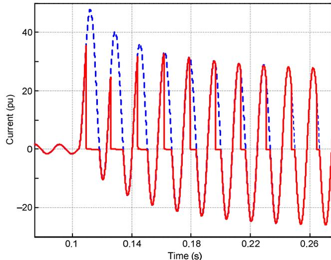
Fig. 15. A-phase CT saturation at Terminal R: ratio current (dashed line) and secondary CT current (solid line).
