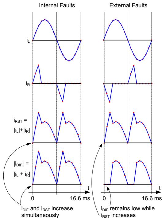
Fig. 20. External fault detection principle.
