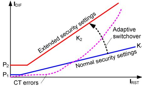
Fig. 2. Adaptive percentage differential characteristic.
