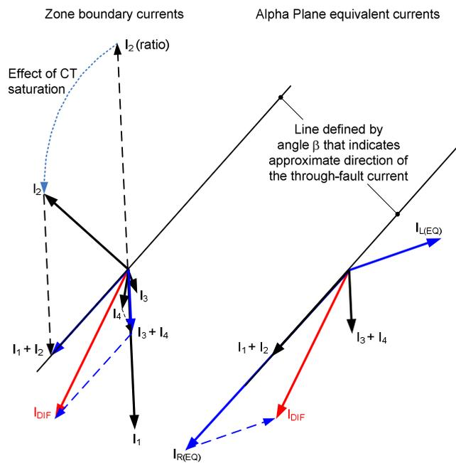
Fig. 12. Current phasors in Example 2, assuming the 87L scheme measures all zone boundary currents individually but the remote relay is provided with partial differential and partial restraining signals only, instead of individual local currents.
