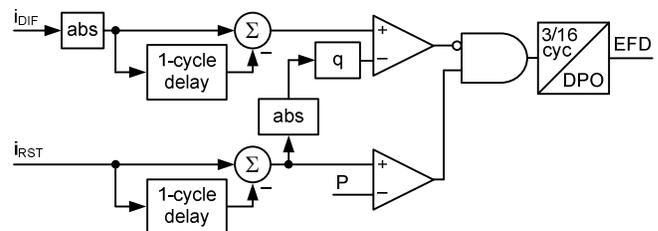
Fig. 22. External fault detector logic.
