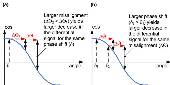
Fig. 28. Larger misalignment impacts dependability more for the same phase shifts between the internal fault currents (a). Larger phase shifts between internal fault currents lead to greater impact of misalignment (b).
