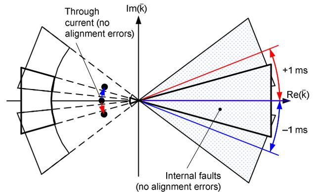
Fig. 4. Impact of current alignment errors on the Alpha Plane.
