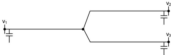
Fig. 30. Lumped parameter three-terminal line model.
