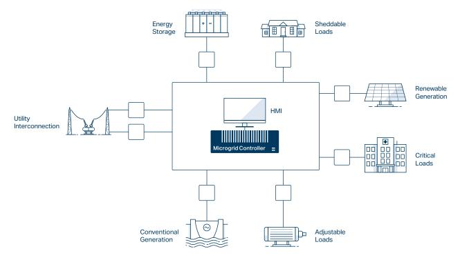
**Incorporate All Assets**—SEL microgrid control systems are capable of protecting and controlling many types of distributed energy resources.
