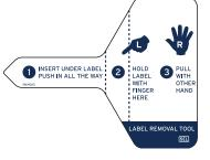
Use the label removal tool to remove labels from the front-panel pockets.
