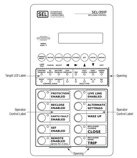
Figure 1 Typical SEL-351P-3 Configurable Label Areas
