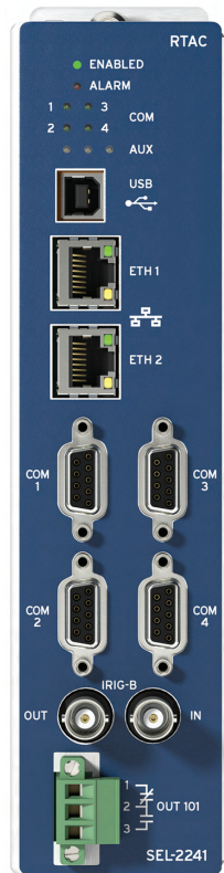
Figure 1 SEL-2241 RTAC Front Panel, Copper Ethernet
