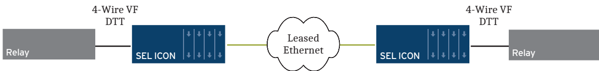
Figure 7 Transporting an Analog DTT Circuit Over a Leased Ethernet Network
