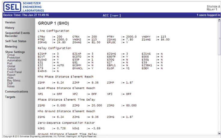
A built-in web server provides easy access to settings, relay status, metering, and event data.
