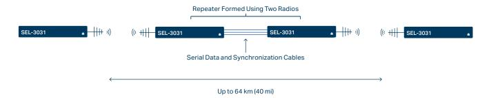
You can connect SEL-3031 radios back-to-back to create a repeater. The repeater configuration can extend the length of a link or maintain radio contact when there is an obstacle between two substations.
