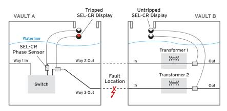
Apply SEL-CRs to outgoing ways of switches and transformers to determine if the fault is beyond the installed (or monitored) location.
