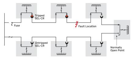
SEL-CRs identify the faulted cable section within a loop of pad-mounted transformers that contain a normally open point.
