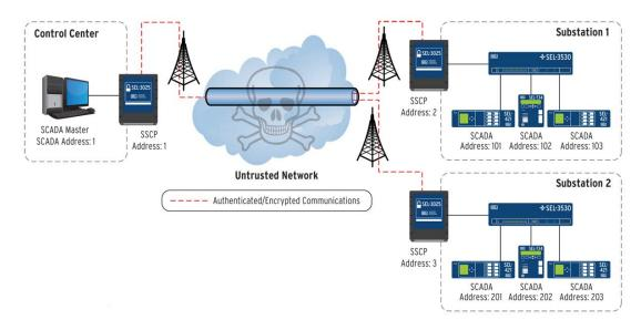
Remotely manage the control center SEL-3025 through a nonintrusive HTTPS interface. If Ethernet is not available to the substation, manage all others through the established secure serial interface.
