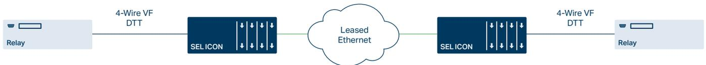
Transporting an analog DTT circuit over a leased Ethernet network.
