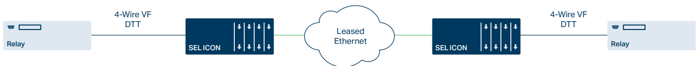
Transporting an analog DTT circuit over a leased Ethernet network.
