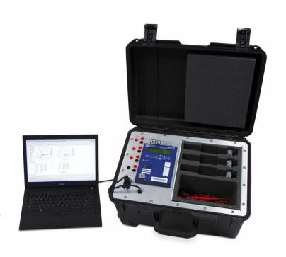
Because the meter is preconfigured, it does not require any settings. Preprogrammed values include trending of: energy and demand; minimum, maximum, and average voltage and current; power factor; harmonics; flicker; voltage sags, swells, and interruptions; and imbalance.
