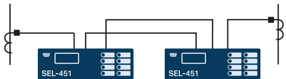
Figure 4 Using Two Cross-Connected SEL-451-5 Relays to Provide Primary and Backup Protection for Two Feeders
