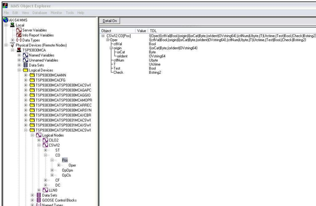
Fig. 7. Control operation sniffing through MMS client
