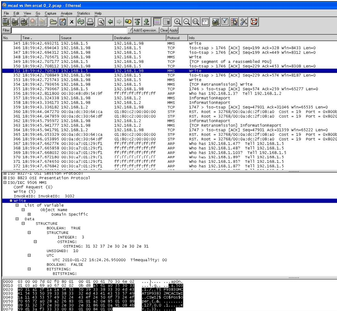
Fig. 6. Control operation sniffing through Ethernet analyzer
