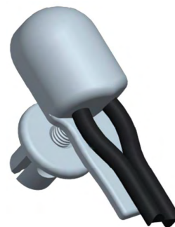
Fig. 2. Fiber-optic point sensor used in the test.
