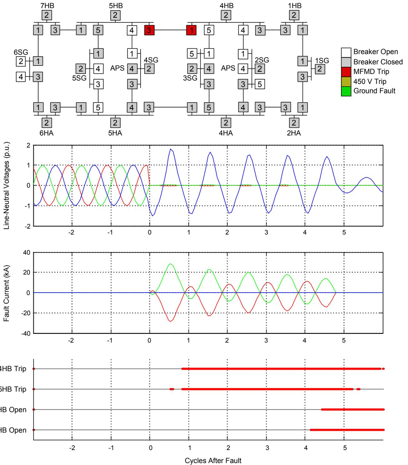
Fig. 14. Backup Protection Clearing a Phase-Phase-to-Ground Bus-Tie Fault
