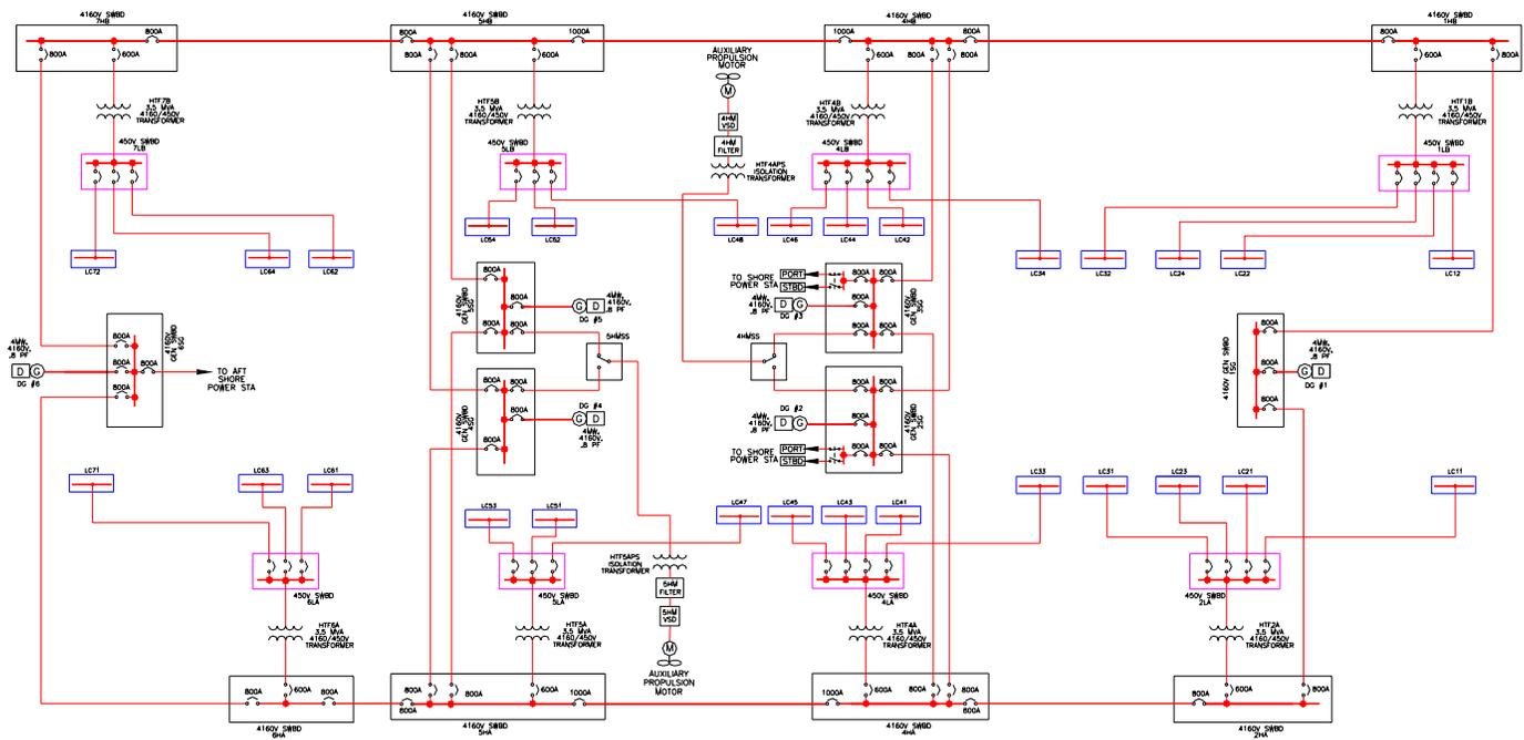
Fig. 2. LHD 8 Electric Plant Single-Line Diagram
