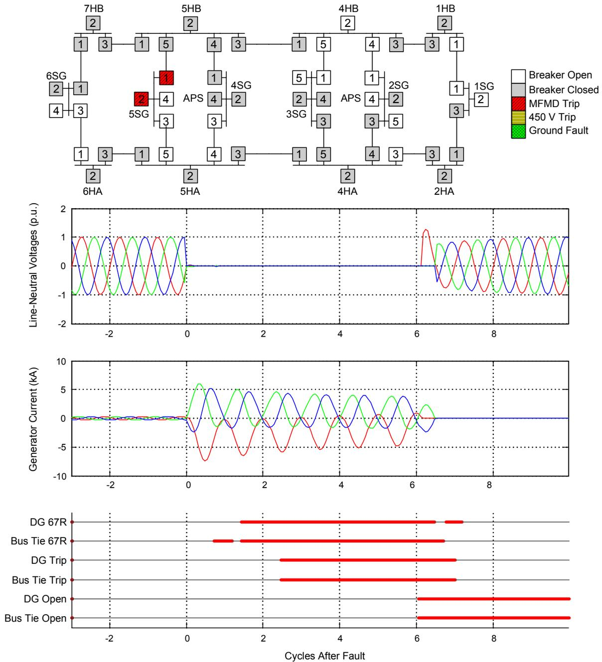
Fig. 20. Detecting a Bus-Bar Fault With Single-Ended Directional Relays
