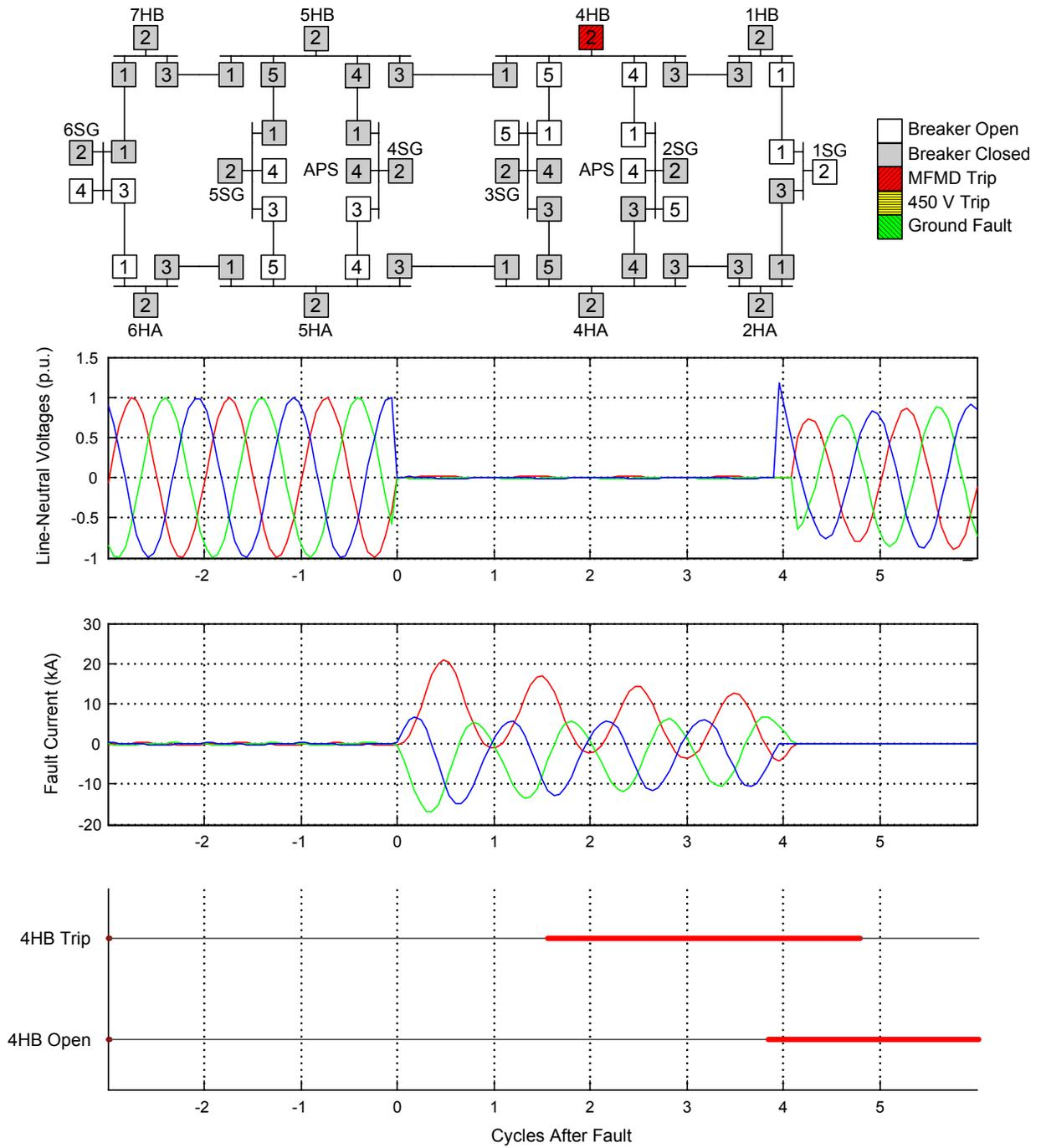
Fig. 16. Clearing a Three-Phase Fault at a Load Center (Primary Side)
