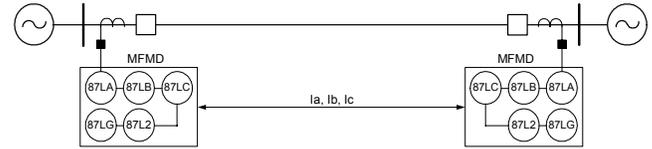
Fig. 6. Typical Line Current Differential Scheme
