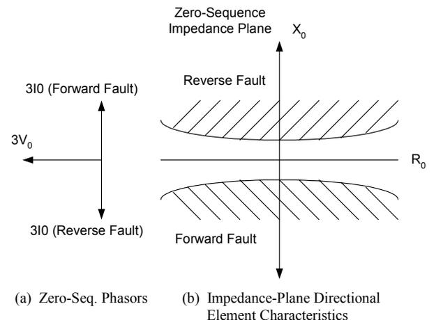
Fig. 10. Ground Directional Element Characteristics
