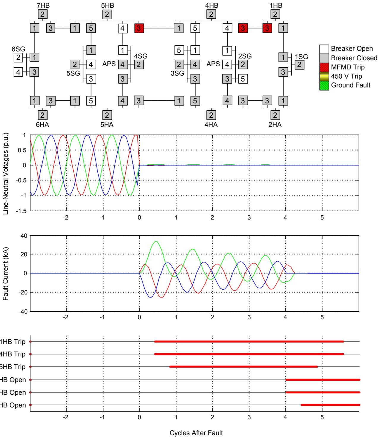
Fig. 15. With Communications Lost, Backup Protection Can Trip for Out-of-Section Faults
