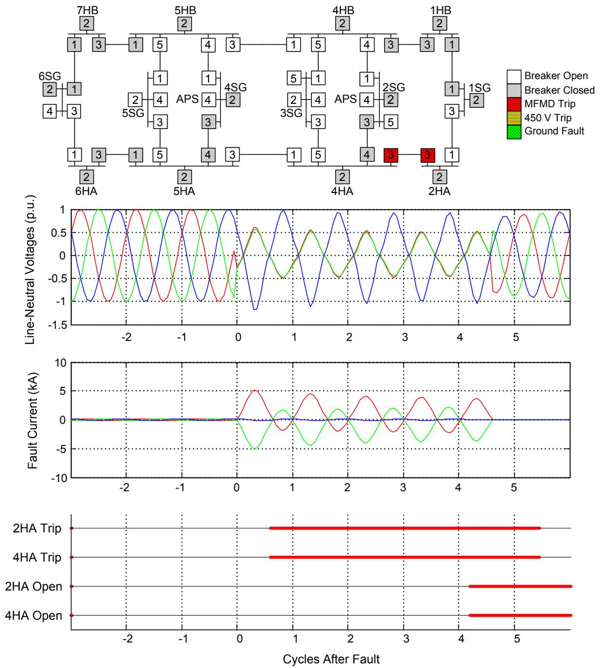
Fig. 13. Isolation of a Phase-to-Phase Fault on a Bus-Tie Cable
