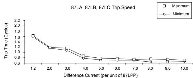
Fig. 8. Operating Speed for Various Fault Levels
