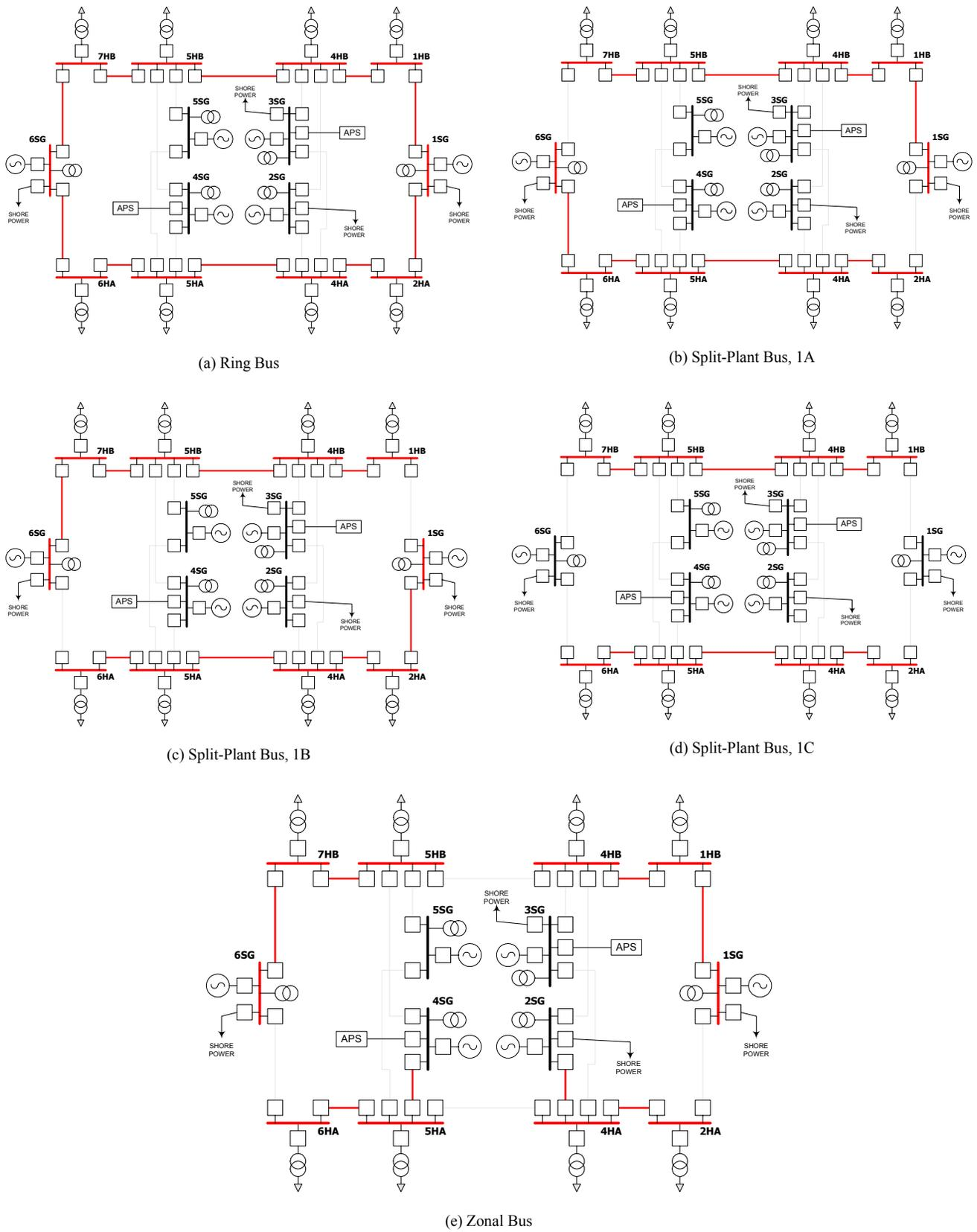
Fig. 3. LHD 8 Standard Electric Plant Configurations
