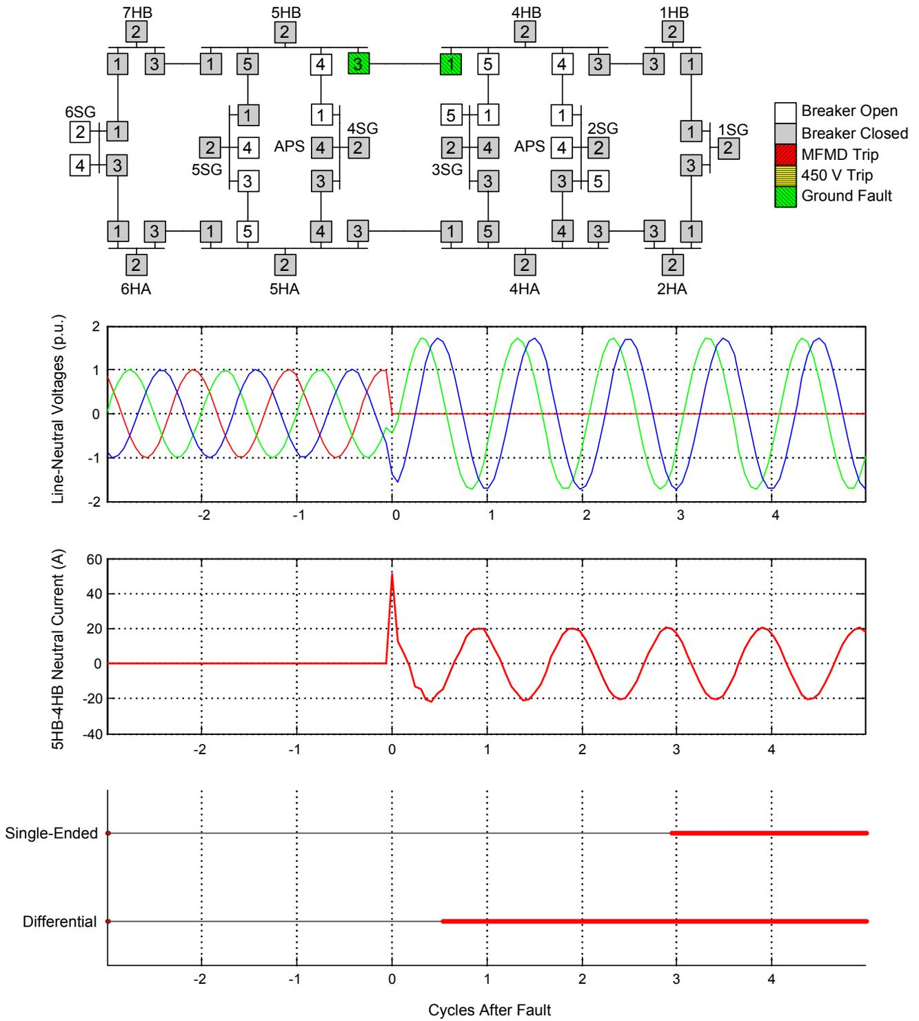
Fig. 18. Differential Detection of a Single-Line-to-Ground Fault
