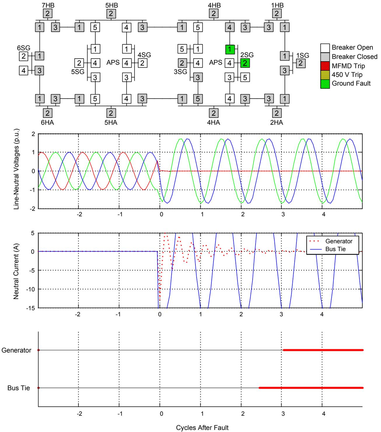
Fig. 19. Cooperative Detection of a Bus Bar Single-Phase-to-Ground Fault
