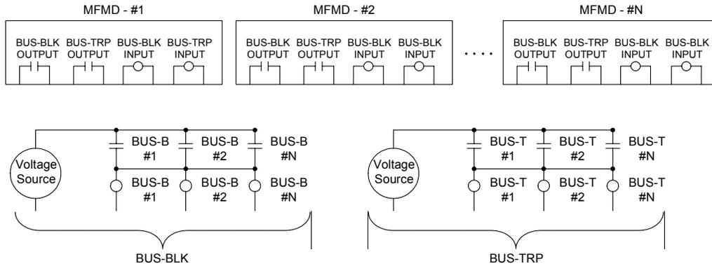
Fig. 12. Bus Block, Bus Trip Wiring Diagram
