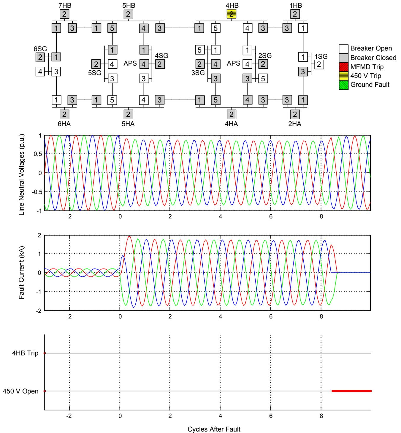
Fig. 17. Low-Voltage Protection Clears a 450 V Fault
