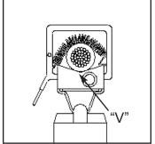
Position indicator so the cable rests in the molded "V" of the phase sensor housing. Using switch stick, close
