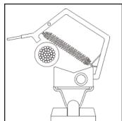
Open core. Using a switch stick and a pulling motion position the MB core around the cable.
