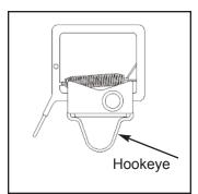
Step 1. Using hotstick grasp indicator at hookeve on face of indicator.
