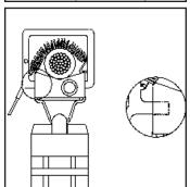
Step 4. Be sure core is properly closed and mated. Position face of indicator for easy viewing. Remove hotstick. Installation complete.
