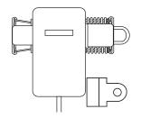
Ensure that the conductor is energized and the minimum load current has been present for at least three minutes. Hold the CRSRTT tool against the bottom right side of the housing for at least 15 seconds. Remove the tool to complete the trip or reset process.
