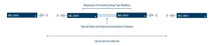
You can connect SEL-3031 radios back-to-back to create a repeater. The repeater configuration can extend the length of a link or maintain radio contact when there is an obstacle between two substations.
