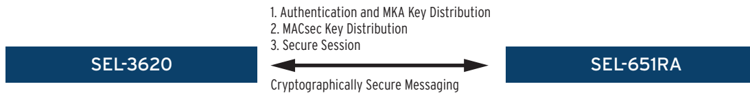
Figure 12 Layer Two Tunnel Establishment
