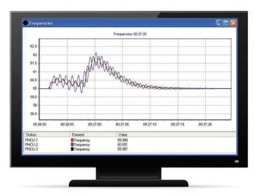
The SEL-487E exceeds the IEEE C37.118 standard with up to 50 messages per second at 50 Hz or up to 60 messages per second at 60 Hz.
