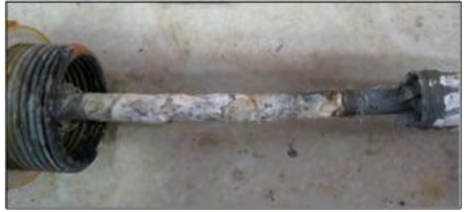
Fig. 18. A failed FO splicing box showing the rusted stand broken from the base and aluminum tube corrosion that caused pressure on fiber, high-signal attenuation, and failure of the communications system
