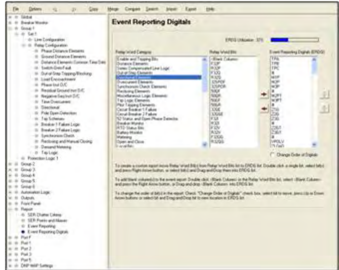
Fig. 14. Example of setting recording digitals for a disturbance recorder
