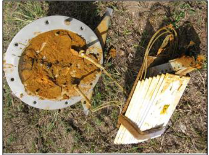
Fig. 44. A failed FO splicing box showing that the rusted stand has broken from the base
