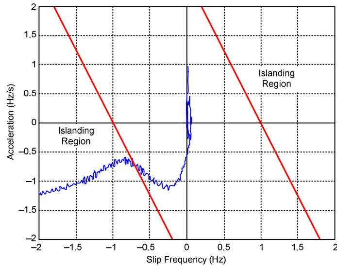
Fig. 9. The operating point enters the islanding region for import power exchange
