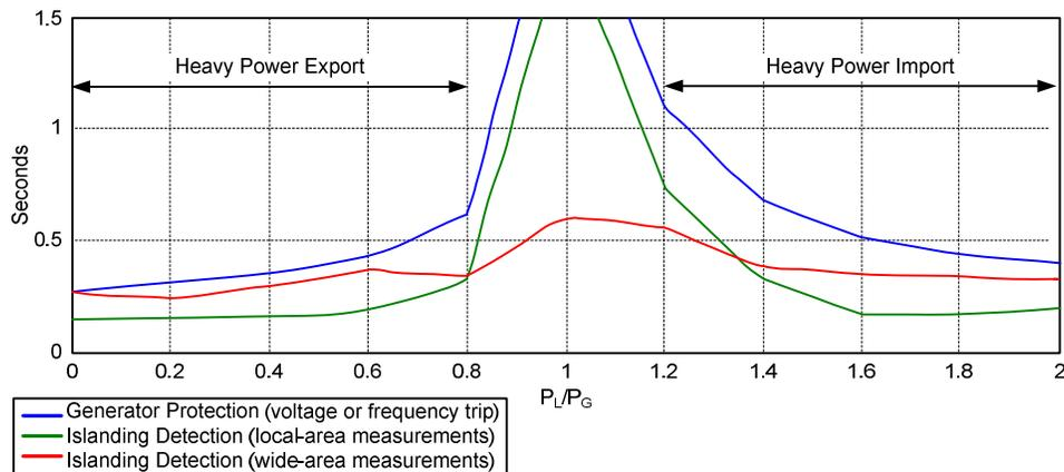
Fig. 12. Operating times of generator protection and local- and wide-area islanding detection schemes for different power exchange conditions
