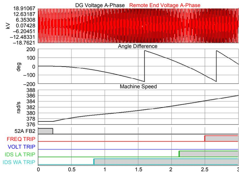
Fig. 10. The IDS\_WA scheme detected the islanded condition for minimal power exchange
