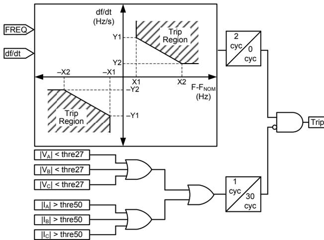
Fig. 2. Islanding detection scheme using local measurements
