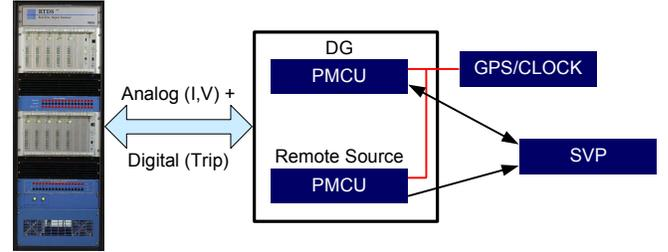
Fig. 5. Test system to verify the operation of the islanding detection schemes
