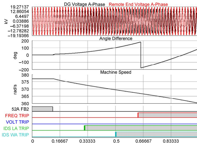
Fig. 8. Local-area measurement-based elements detected the islanded condition for import power
