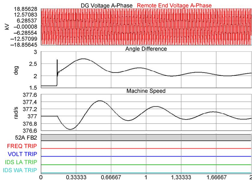
Fig. 11. Islanding detection elements are stable during induction motor switching
