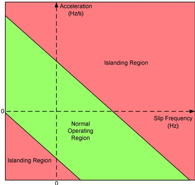
Fig. 3. Islanding detection characteristic using wide-area measurements
