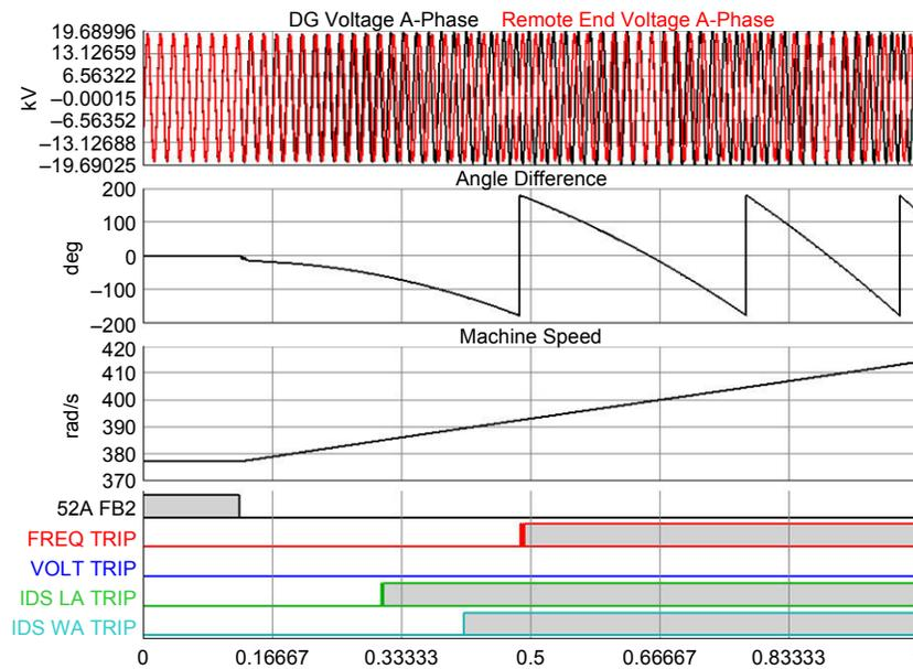
Fig. 7. Local-area measurement-based elements detected the islanded condition for export power
