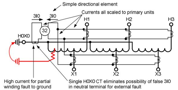
Fig. 5a. Traditional Current Polarized Directional REF Scheme
