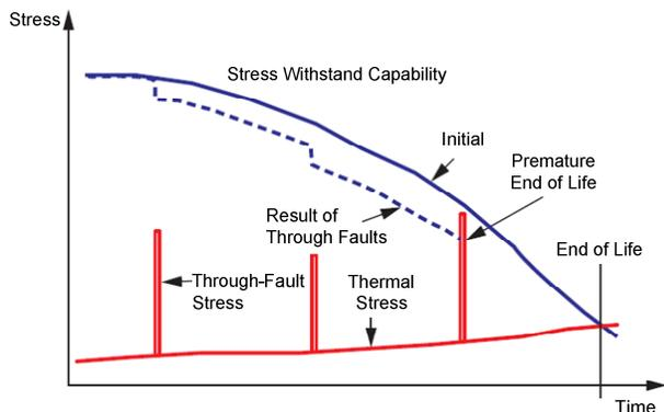
Fig. 6. Combined Effect of Thermal Stress and Through Fault on End of Life
