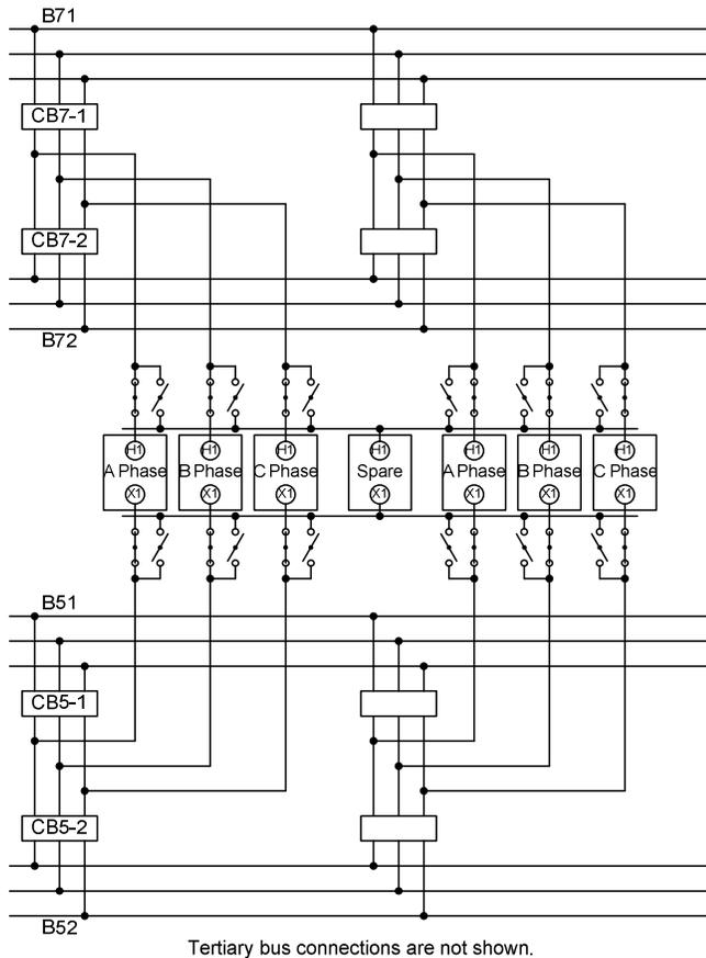
Fig. 1. Two Three-Phase Banks With Shared Spare
