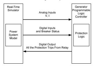
Fig. 16. RTDS and Test Model Connection
