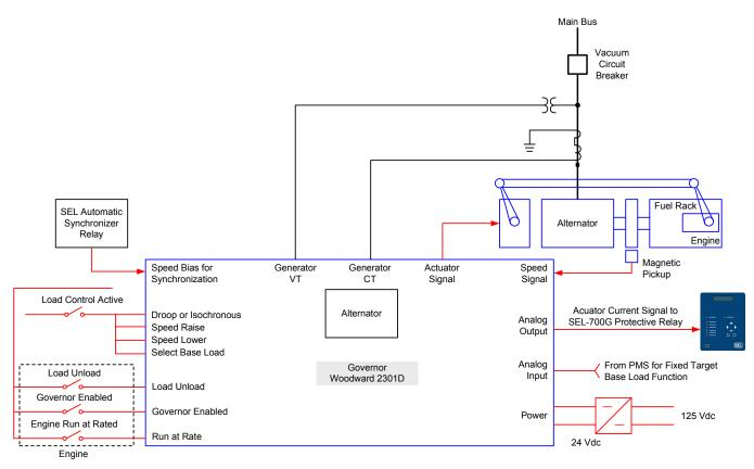
Fig. 13. Typical Woodward Governor and Controls
