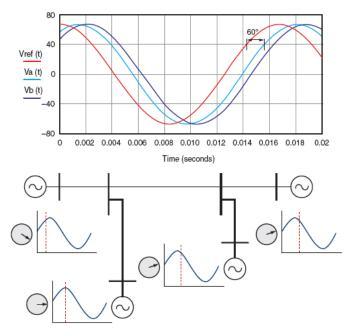
Fig. 6. Synchrophasor Measurement
