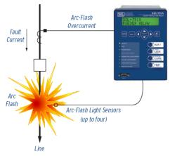
Fig. 9. High-Speed Arc-Flash Detection
