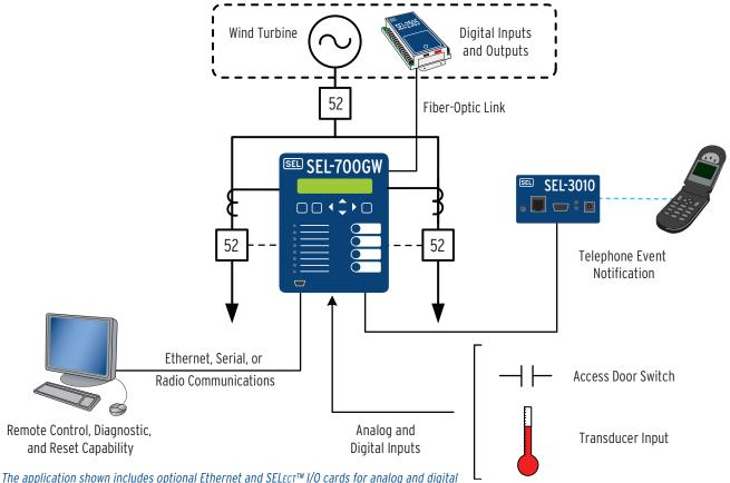
The application shown includes optional Ethernet and SELεct™ I/O cards for analog and digital I/O. The SEL-3010 Event Messenger and SEL-2505 Remote I/O Module are sold separately.
