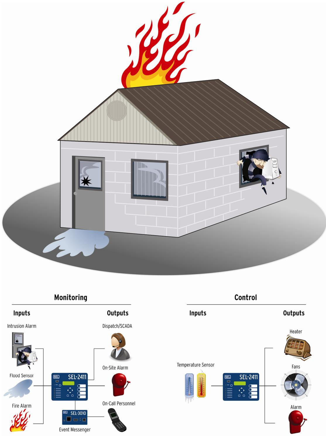
Figure 1 Building Monitoring and Control
