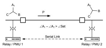
Figure 1 Relay-to-Relay Synchrophasor Communications and Logic
