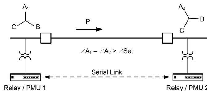
Figure 1 Relay-to-Relay Synchrophasor Communications and Logic
