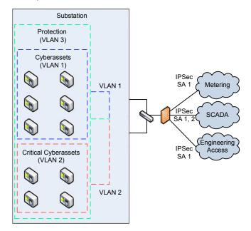
Fig. 4. IPSec VPN operating with a VLAN and a firewall
