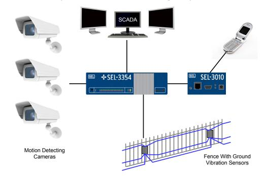
Figure 1 Physical Surveillance System
