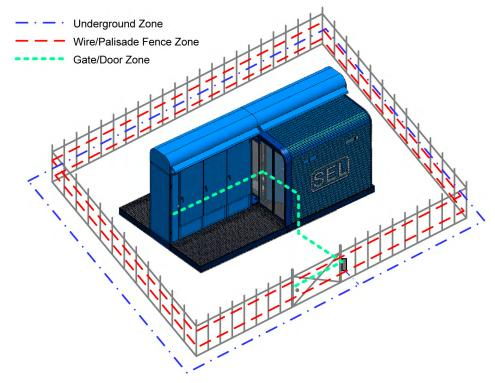
Figure 2 Typical Perimeter Security Monitoring
