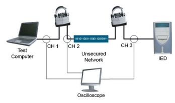
Fig. 7. Test Configuration
