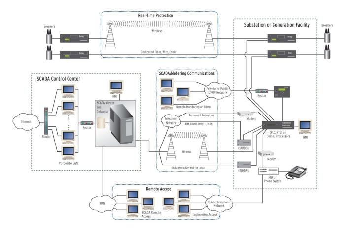
Fig. 1. Electric Utilities Communications Links
