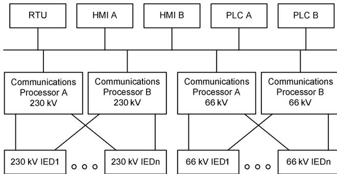
Fig. 6. Portage la Prairie South Fully Redundant Control System Architecture
