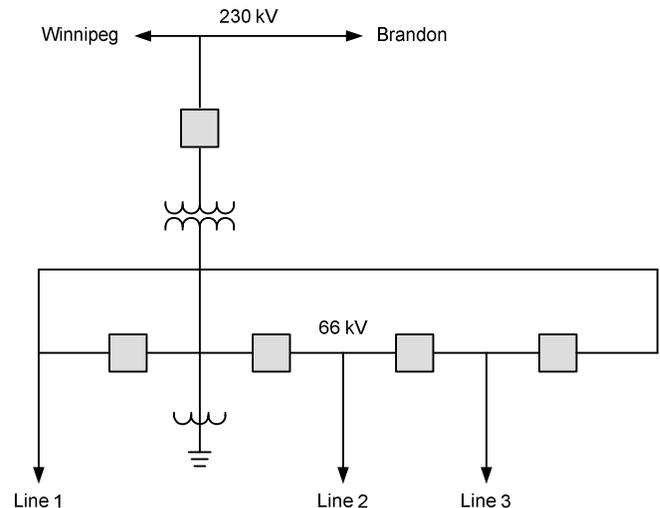
Fig. 2. Portage la Prairie One-Line Diagram Prior to the Upgrade
