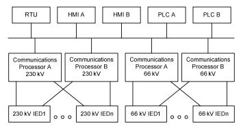
Fig. 6. Portage la Prairie South Fully Redundant Control System Architecture
