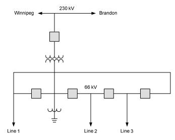
Fig. 2. Portage la Prairie One-Line Diagram Prior to the Upgrade
