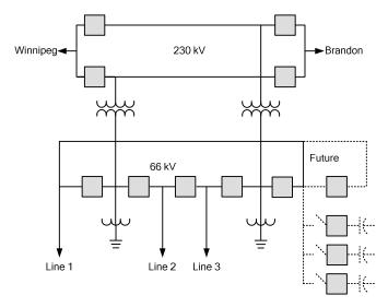
Fig. 3. Portage la Prairie One-Line Diagram After the Upgrade
