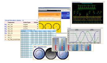
Fig. 11. Web Parts for Interfacing to the Web-Based Data Pool
