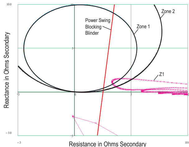
Fig. 19. Impedance Plan Plot of High-Load Power Swing Blocking Scheme
