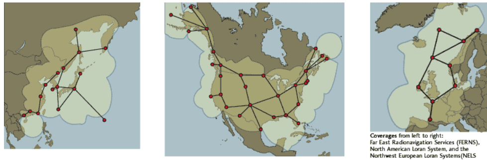
Fig. 26. LORAN-C Coverage Areas, (Picture Courtesy of Megapulse) [9]
