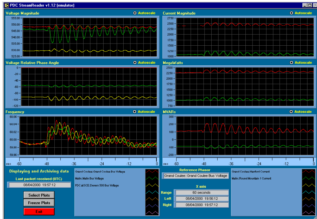
Figure 26 StreamReader Real-Time Data Display Showing Sustained System Oscillation After a Line Outage
