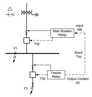
Fig. 10. Fast Bus Trip Scheme
