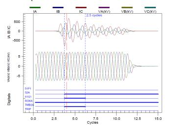
Fig. 18. Feeder Breaker Relay Data During Commissioning Tests
