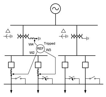
Fig. 22. Simplified One-Line Diagram of REF Operation
