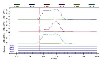
Fig. 9. Differential Relay Operate and Restraint Currents After Settings Change
