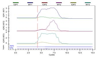
Fig. 6. Differential Relay Operate and Restraint Currents for Through Fault
