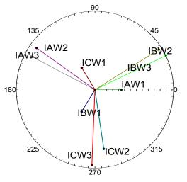
Fig. 23. Winding Currents From Differential Relay Match Expectations
