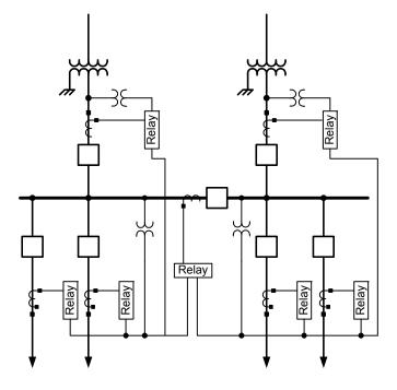
Fig. 16. One-Line Diagram of New Substation
