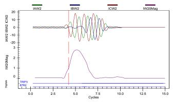
Fig. 8. Low-Voltage Winding and Zero-Sequence Currents for Through Fault
