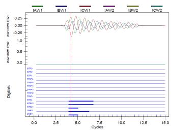
Fig. 21. CTs Shorted on Differential Relay Low-Side Winding
