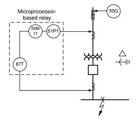
Fig. 1. Ground Overcurrent Protection for Delta-Connected Transformer Winding
