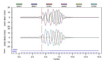
Fig. 5. Transformer Differential Relay Trips for an Out-of-Zone Fault
