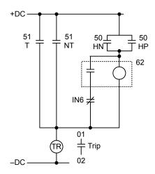
Fig. 13. Main Breaker Relay Trip Logic
