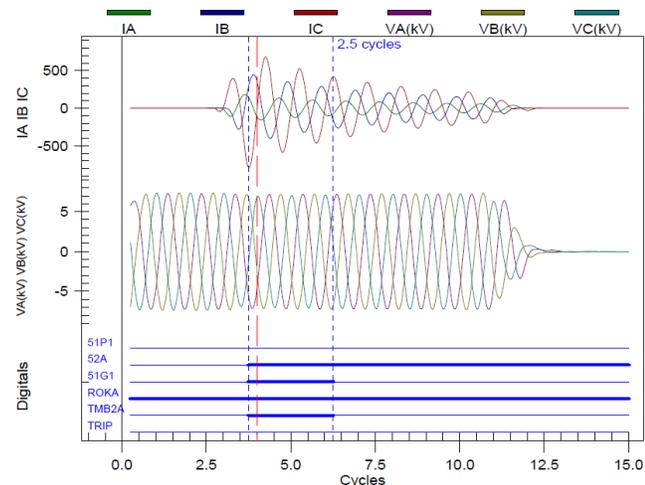
Fig. 18. Feeder Breaker Relay Data During Commissioning Tests
