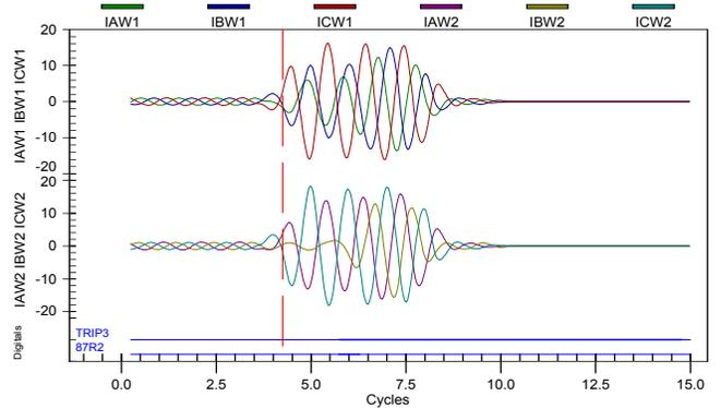
Fig. 5. Transformer Differential Relay Trips for an Out-of-Zone Fault
