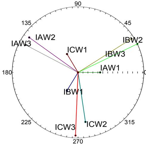
Fig. 23. Winding Currents From Differential Relay Match Expectations
