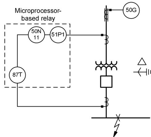
Fig. 1. Ground Overcurrent Protection for Delta-Connected Transformer Winding
