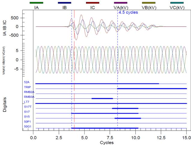
Fig. 17. Bus-Tie Breaker Relay Trips During Commissioning Tests
