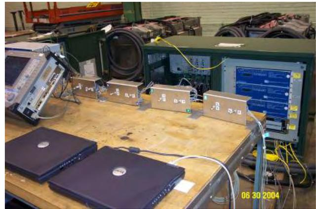
Fig. 5. Factory testing of protection schemes and communications
