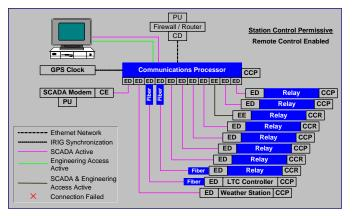
Fig. 7. HMI Screen Showing Status of Substation Communications and Control Status [15], [16]
