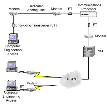
Fig. 5. Adding Serial Encrypting Transceivers Provides Data Security
