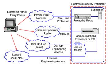
Fig. 2. Typical Modern Substation Network
