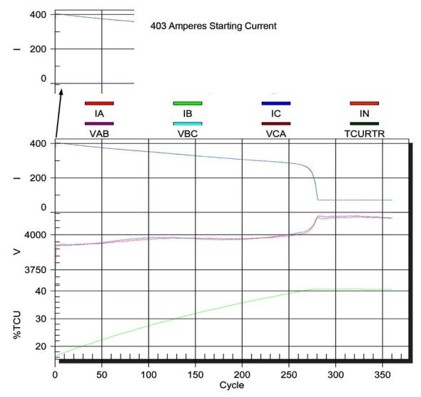
Fig. 3. Example of Graphical Motor Start Report
