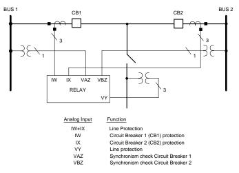
Fig. 3. Example of a Relay Configuration Provided by the Manufacturer
