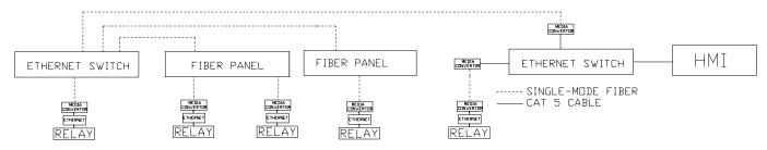
Fig. 15. Ethernet Communication Network
