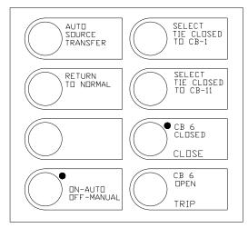
Fig. 12. Automatic Transfer Pushbuttons
