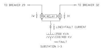
Fig. 4. Fault on Remote Station Bus or Transformer
