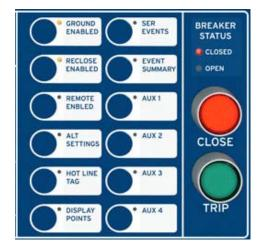
Fig. 11. Local Breaker Control Panel
