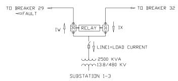
Fig. 5. Fault on Line Protected by Breaker 30
