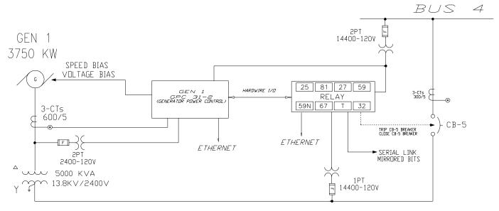
Fig. 14. Hardware Interconnections for Generator Controls
