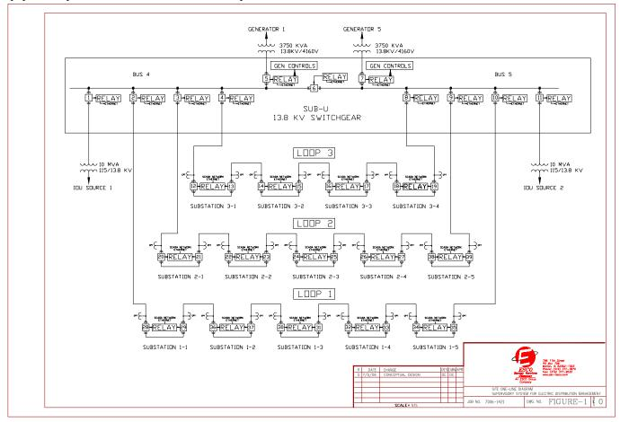
Fig. 1. South Electrical One-Line Diagram
