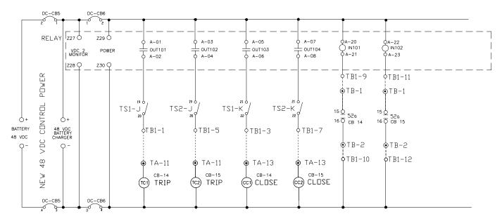
Fig. 9. DC Breaker Control Schematic
