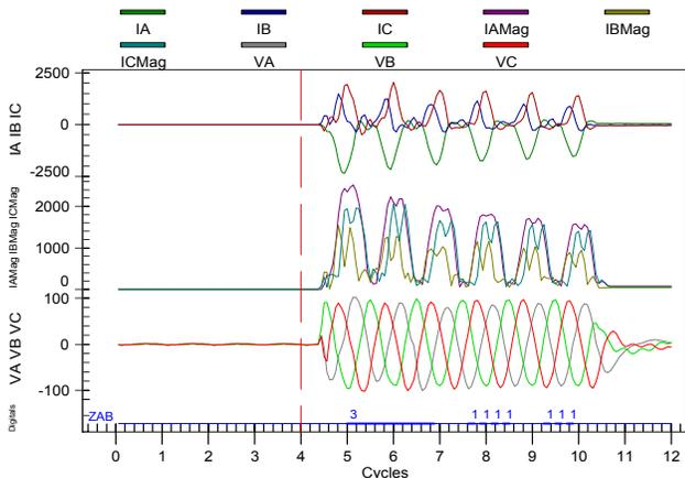
Fig. 18. Raw Data From Local Relay During Reclose
