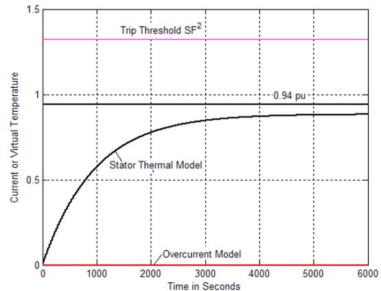
Fig. 11 Warm Up With a 0.94 pu Load Current
