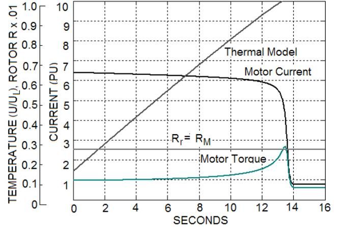
Fig. 7 Motor Starting Current With  $I^2t$  Temperature Response
