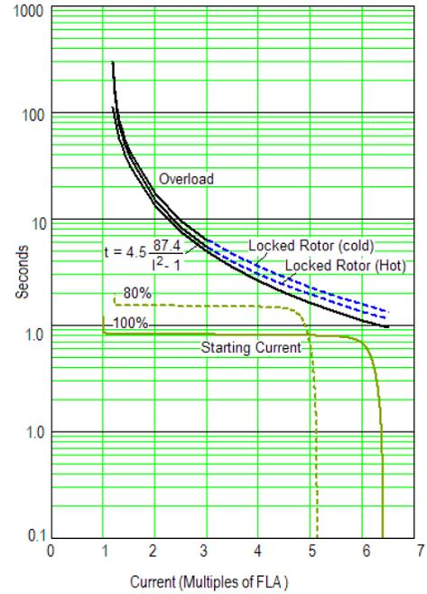
Fig. 10 Coordination of Overcurrent Relay Model With Thermal Limit Curve
