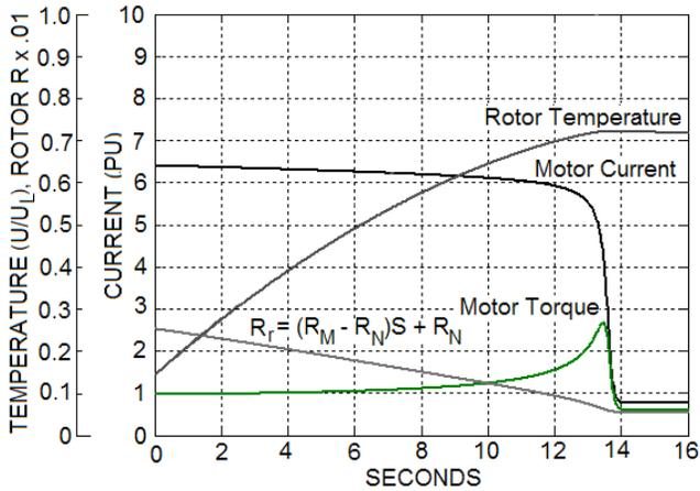
Fig. 6b Motor Starting Current, Motor Torque,  $R_r$ , and Temperature
