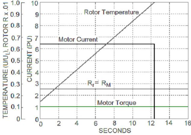
Fig. 6a Locked Rotor Trip. At Locked Rotor  $S=1$ ,  $R_r = R_M$
