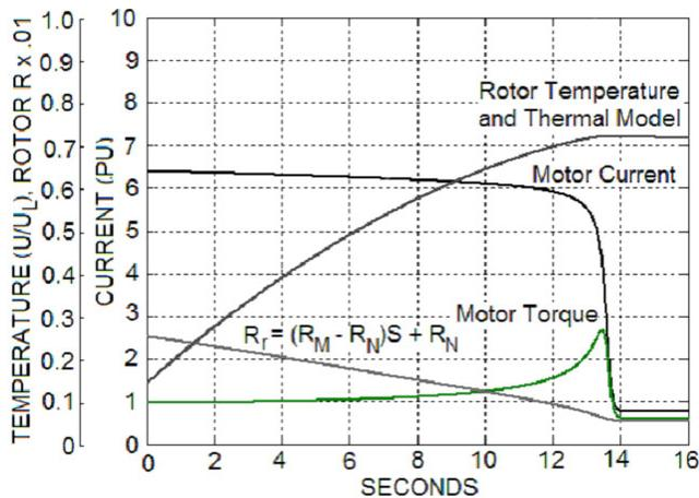
Fig. 8 Motor Starting Showing Thermal Model Emulating the Rotor Temperature
