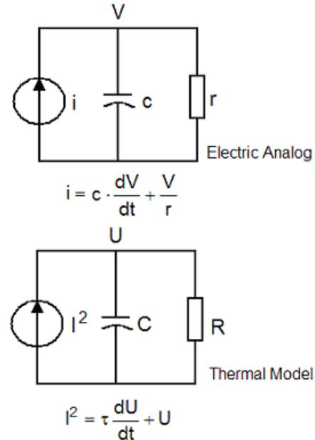
Fig. A1 The Electrical Analog Circuit of the Thermal Model
