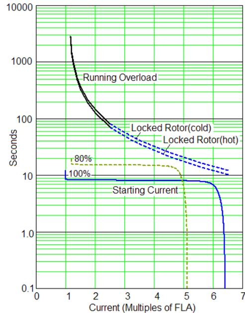
Fig. 1 7000-hp, 900-rpm Motor Thermal Limit Curves
