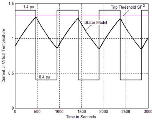
Fig. 12 Stator Model Temperature Response to Cyclic Load
