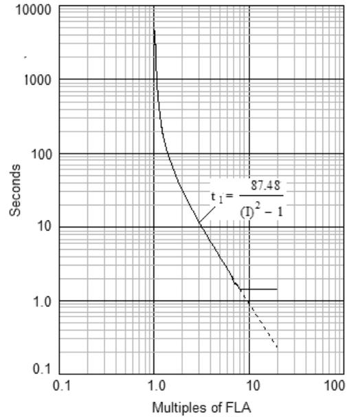
Fig. 2 Time-Current Curve for Adiabatic Derivation
