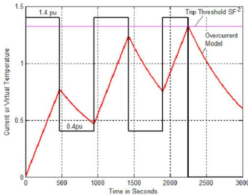
Fig. 13 Overcurrent Model Response to a Cyclic Load
