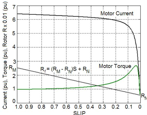
Fig. 4 Motor Current, Torque, and Rotor R Plotted Versus Slip
