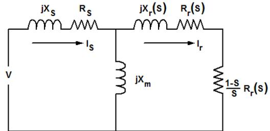
Fig. 3 Steinmetz Motor Equivalent Circuit
