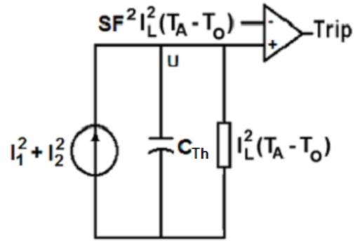
Fig. 9 Stator Thermal Model
